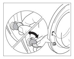
To disable this device and restore the possibility of closing the door, rotate the button counterclockwise until the groove is vertical.
